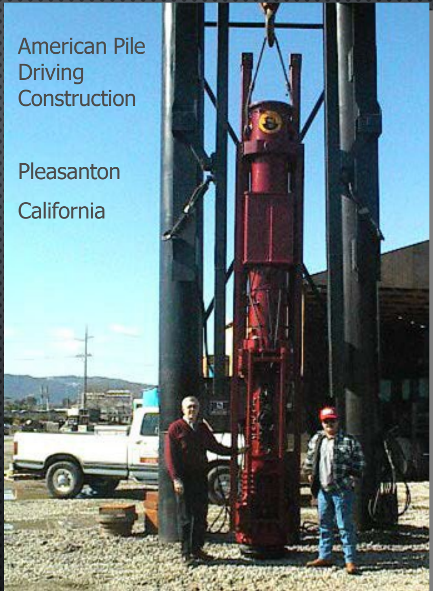
APE D30 without sound shielding
