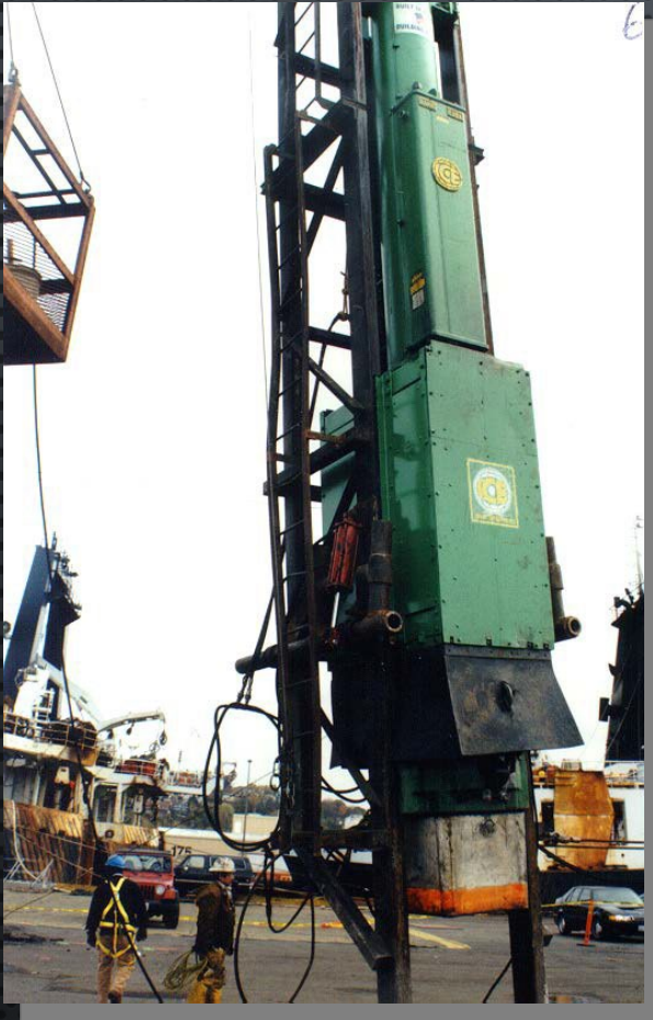
ICE 100S with sound shielding (ICE Seattle)
